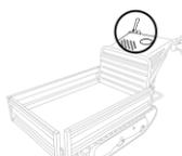
fig.16 Accelerator control lever
