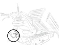
fig.17 Gear control lever
