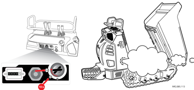
fig. 31– Verification of plugs preheating system
