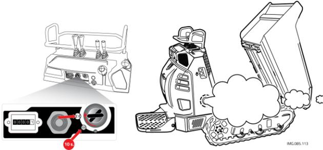
fig. 31– Verification of plugs preheating system
