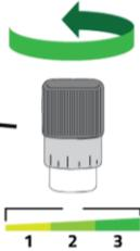
Loosen the potentiometer to bring the engine back to the right speed
