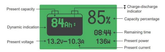
For example, the below LCD display means:
