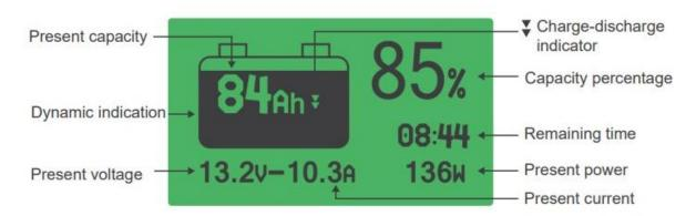
For example, the below LCD display means:
