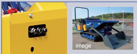
Auxiliary third valve for attachment like self loader etc.
